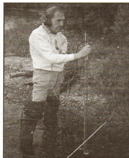
At left, a volunteer with the local self-help Secchi disk water clarity test program sponsored by the Michigan Lakes and Streams Association prepares to lower the disk into the water. At right, Walt Nielsen measures a tributary's stream flow with a pygmy current meter in a program sponsored by the Leelanau Watershed Council.
