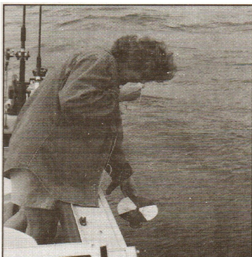
At left, a volunteer with the local self-help Secchi disk water clarity test program sponsored by the Michigan Lakes and Streams Association prepares to lower the disk into the water. At right, Walt Nielsen measures a tributary's stream flow with a pygmy current meter in a program sponsored by the Leelanau Watershed Council.
